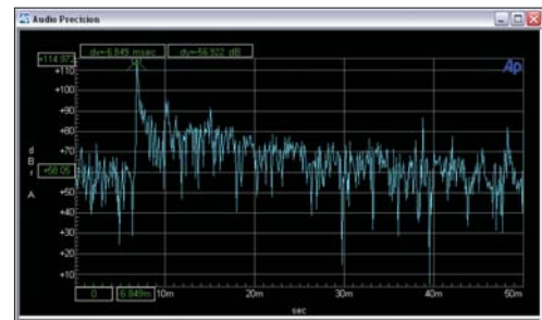
Loudspeaker impulse response graph, showing a 6.6 ms delay before the impulse peak.
